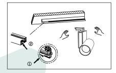
After finishing assembly,rotate to the desired position and turn on
